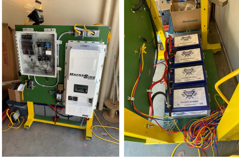
Figure 1: On the left, a view of the micro-grid system controller-inverter. The front panel also includes a number of circuit breakers and power outlets. On the right, the four Lithium-ion batteries providing 4.8 kW-hr of energy storage.
