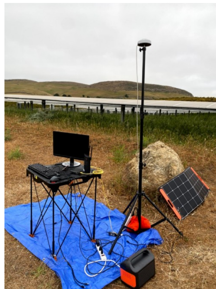
Figure 3: Complete Total Sky Imager (TSI) system tested on May 14, 2021. System consists of a Raspberry Pi, TSI camera, LTE router, lithium battery, and solar panel.
